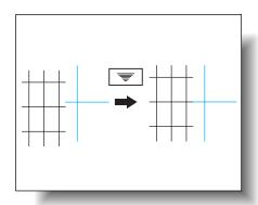
11 If the lines are shifted as shown at the right, touch [Y], and then touch to specify the desired positive adjustment for "Y" (between +1 dot and +6 dots).
